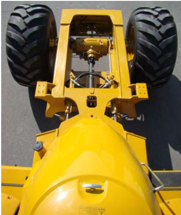
The MultiChassis seen from above. Here the 912D MultiChassis, ready for add-on-tools.
