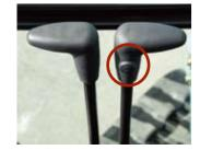
The travel lever is fitted with a button for easy switching to Hi-Mode travel.
