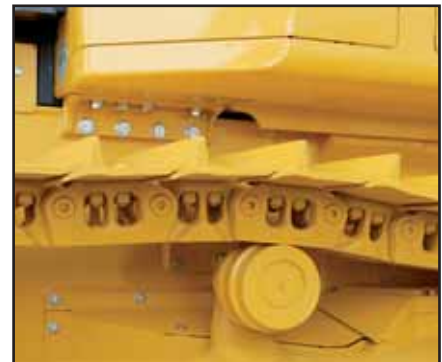
Komatsu Parallel Link Undercarriage System (PLUS)
