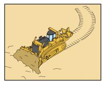
When dozing and turning, the ECMV automatically controls the stroke ratio of the steering clutches and brakes, depending on degree of load, enabling smooth dozing and turning.
