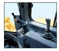
**Blade and ripper control joystick** The blade and ripper control joysticks have an ergonomic design and allow long operator work shifts with fine blade control.
