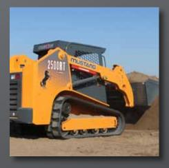
ANTISTALL TECHNOLOGY A monitors and adjusts the hydrostatic drive pump, resulting in tractive effort of 11,840 lbs. (5371 kg) on the 1750RT, 12,359 lbs. (5606 kg) on the 2100RT, and 14,317 lbs. (6494 kg) on the 2500RT.
