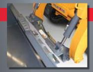
MULTI-TACH® SYSTEM standard on all models is this universal-style attachment mounting system that is compatible with most allied attachments.
