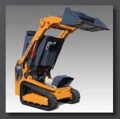
SERVICEABILITY A is made easy with a large gas-spring assisted engine cover and tiltable ROPS/FOPS assembly. Patented tilt-out foot pod allows for best-in-class foot well cleanout and easy access to components under the cab.
