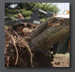
**HYDRAULIC SYSTEM** with flow up to 37.4 gpm (141.6 L/min.) on the 2500RT delivers high performance and fast cycle times. Lift cylinders incorporate cushioning for smoother operation when lowering the lift arm.
