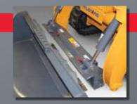
POWER-A-TACH® SYSTEM A optional on all models, users quickly install and remove attachments electronically, leaving the seat only to connect auxiliary hydraulics.
