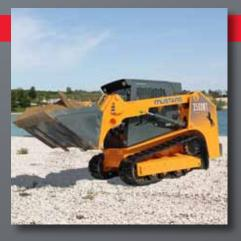
DEDICATED, WELDED TRACK LOADER CHASSIS A adds durability and aids in superior weight distribution, which enhances stability, grading and tractive effort.
