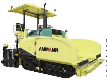
Tracked machine with rubber pads; automatic tensioning device system with grease accumulator. Hydrostatic transmission with two variable flow rate pumps which feed two motors with two displacements directly fastened to the planetary gearboxes which operate the tracks. Mounted on each pump, an electronic and proportional control gives a progressive start and stop,
