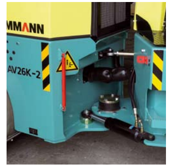
Life time lubricated central articulation joint
