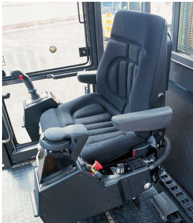
Sliding & rotating seat with integrated control instruments
