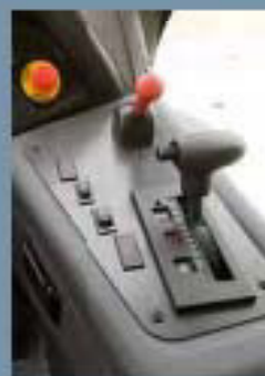
↑ Tarate in acciaio inossidabile Gear lever and parking brake
