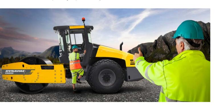
Tools: A fifth generation Dynapac CA soil compactor, equipped with Compaction Optimizer, incorporating Compaction Meter and Compaction Analyzer, with GPS (optional).
