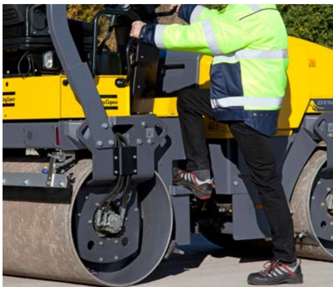
Sturdy handgrips and ergonomic steps enable safe boarding.
