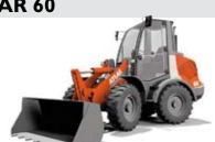
Operation weight 4650 kg 47.5 kW (65 HP) Power Shovel capacity 0.85 m<sup>3</sup>
