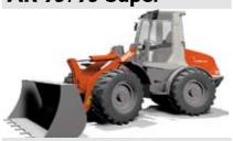
7900 kg / 8100 kg Operation weight 74.9 kW (102 HP) / 92 kW (125 HP) Shovel capacity I.40 - I.60 m<sup>3</sup>
