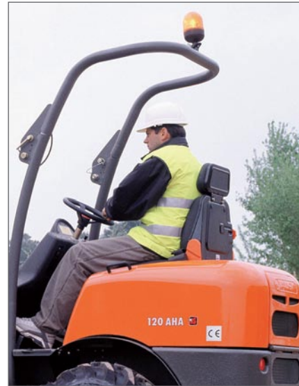
Driving site with folding FOPS structure
