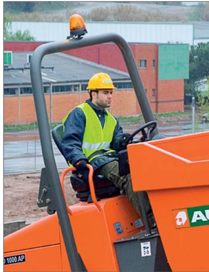
Driving site with folding FOPS structure
