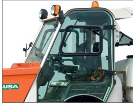
Sound-proof and ROPS/FOPS closed cabin (D 150/175 R, D 201 R & D 600/700/1000 A)
