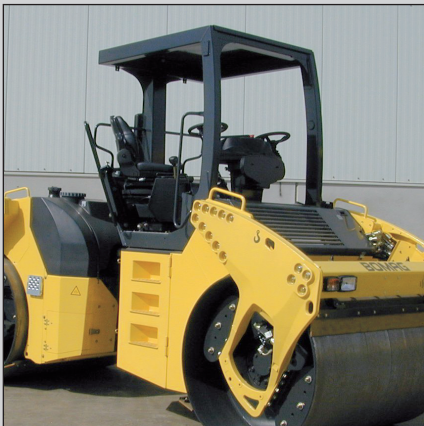
Safety: Operator's platform with rail and ROPS/FOPS.
