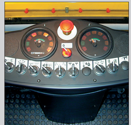
Safety: emergency stop switch and warning lights are centrally located.
