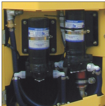
Sprinkler system with two pumps: can be easily switched from the operator's platform.
