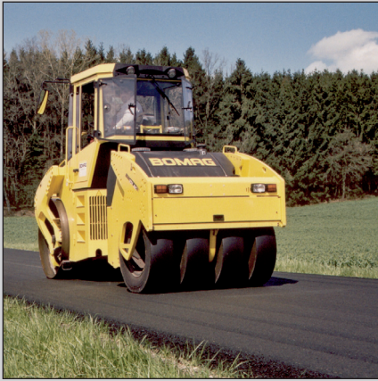
Combination rollers give good surface sealing effect.
