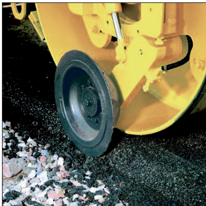
Efficient edge working with cutting disc or pressure rolls.
