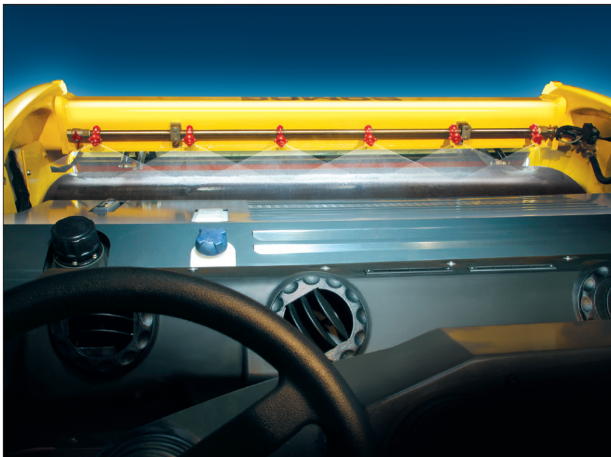
Optimum water distribution with 6 nozzles; a proven system with triple filtering.
