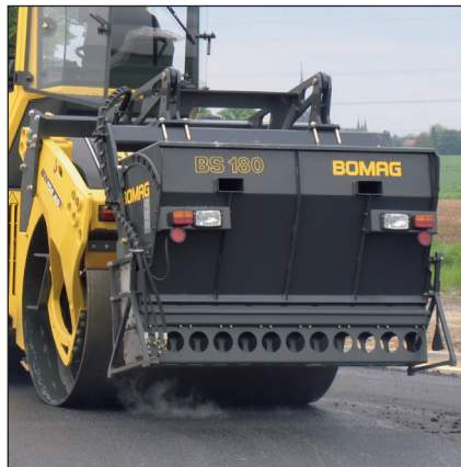
BS 180 precision chip spreader for precise and even coverage.
