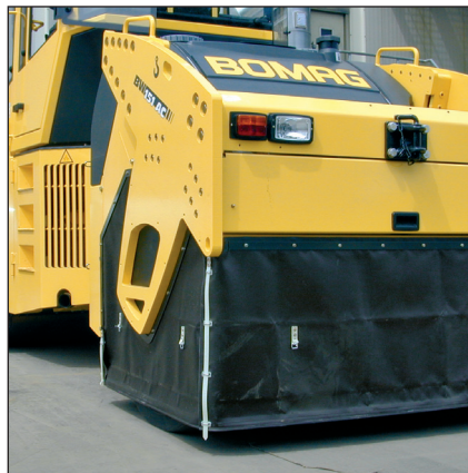
Thermal apron: keeps the tyres on a combination roller warm for longer.
