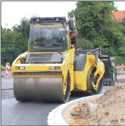
BW 154 AD with split drums; problem-free around bends.
