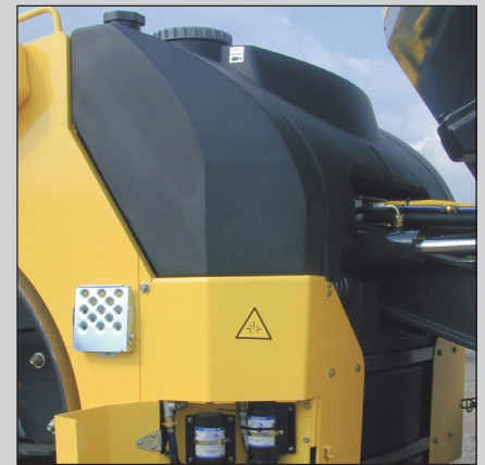
Large water tanks for fewer tank stops.
