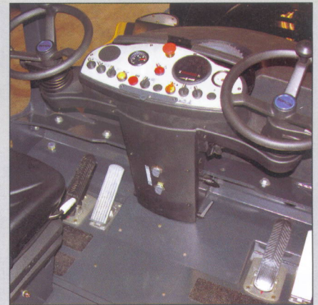
Two complete operator platforms with swivel/sliding seat make work more efficient and give good visibility.
