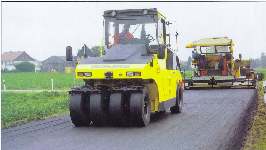
The BW 25 RH is a flexible pneumatic tyred roller for compaction work in asphalt and earthworks.
