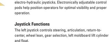
The right joystick controls drawbar, circle and moldboard functions as well as electronic throttle control and manual differential lock/unlock.
