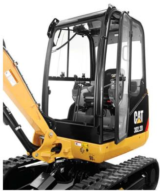
The Cat 302.2D cab is amongst the largest in the industry. The flat cab floor optimizes visibility and increases operator leg room. The ergonomic control layout provides a comfortable, highly productive workspace.
