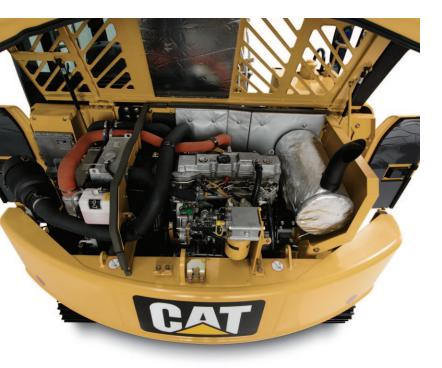
Robust, reliable and easily serviceable are the key attributes of Cat<sup>®</sup> Mini Hydraulic Excavators. Full steel body work panels and protected front linkage lines are routed neatly out of the way of potential damage above the boom. Easy access to all daily service points are accessed through the rear hood and side cover. A 500 hour engine oil change period lowers operating costs and the Cat S•O•S<sup>SM</sup> points assist easy oil sampling for preventative maintenance checks.
