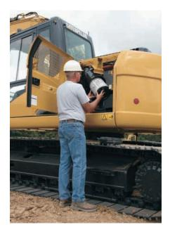
**Ground Level Service.** The design and layout of the 320D LRR was made with the service technician in mind. Many service locations are easily accessible at ground level allowing critical maintenance to get done quickly and efficiently.
