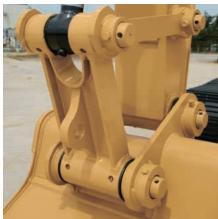
**Bucket Linkage.** The power link improves durability, increases machine-lifting capability in key positions and is easier to use than compared to the previous power link. Lifting from the power link lift eye gives you the optimum lift performance. It allows you to lower the load point, which maximizes the use of the boom cylinders.
