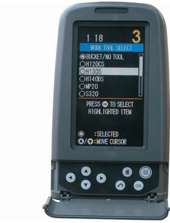
**Auxiliary Hydraulic Options.** Allows you to configure your 320D LRR to meet your work tools needs, while increasing its versatility.
