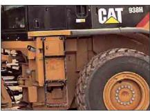
Entry and Exit. A ladder with aggressive tread pattern keeps debris build-up to a minimum. The ladder is at a 5° forward incline for easy entry and exit.
