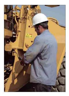
**Ground Level Grease Points.** Grease fittings are grouped on the right side of the machine in two convenient locations thus facilitating easy lubrication of vital components throughout the machine.
