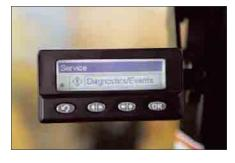
**Cat Messenger.** Messenger offers the comfort of providing real-time, visual feedback on engine and machine operating conditions. It displays information on diagnostic codes, maintenance and system parameters.
