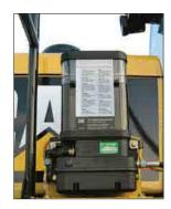
**Hydraulic Service Center.** Transmission oil and hydraulic oil filters are located in the Hydraulic Service Center, behind the hinged, right-side access ladder. The hydraulic oil tank can be drained from this location using the access port.
