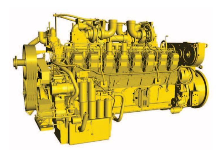
**Engine.** Field-proven Cat® 3516B HD EUI (High Displacement) turbocharged and aftercooled diesel engine delivers high power and reliability in the world's most demanding mining applications. The 3516B is a 16-cylinder, four-stroke design that uses long, effective power strokes for more complete fuel combustion and optimum efficiency.
