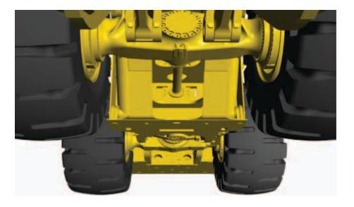
**Torque.** Torque is developed at the wheel, generating less stress and wear on the axle shafts.
