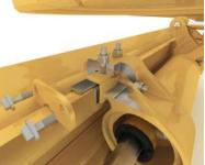
Caterpillar designs motor grader frame and drawbar components to give you performance and durability. The one-piece forged steel circle stands up to high stress loads, and a sacrificial wear system helps keep your service time and costs down.
