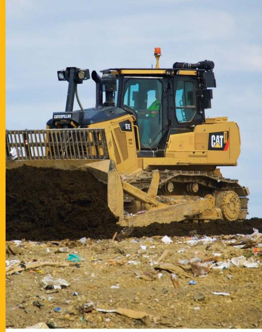
Like all Cat<sup>®</sup> waste handlers, the D7E is a heavy-duty machine with specialized guarding designed just for waste handling applications. Its versatility makes it a powerful and highly maneuverable machine for dozing and compacting waste, as well as an ideal fine grading machine to place just the right depth of cover material.
