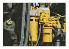
**Electric Priming Pump.** An electric fuel priming pump located on the primary fuel filter base eliminates the need to pre-fill or manually prime filters after a change, eliminating engine contamination.
