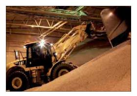
The standard programmable automatic kick-outs provide flexibility and productivity for precise load and dump target heights. Tilt, lift and return-to-dig kickouts are set by positioning the bucket or work tool and setting a rocker switch in the cab.
