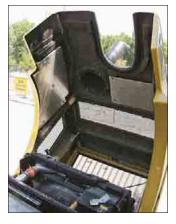
**Cooling System.** Access for clean-out and maintenance is outstanding. The perforated and corrugated grill minimizes debris build-up and swings out for easy cleaning and access to the cooling cores. The full-width air conditioning condenser and oil cooler cores swing out 45° to allow easy cleaning of the rear radiator face. Panels on either side provide access to the front face of the radiator and ATAAC cores for easy cleaning.
