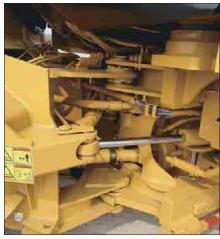
**Spread Hitch**. The distance between the upper and lower hitch plates is important for machine performance and component life. The Cat spread hitch design provides excellent load distribution and bearing life. Both the upper and lower hitch pins pivot on double tapered roller bearings – improving durability by distributing both vertical and horizontal loads over a larger surface area. The wide opening also provides excellent service access.
