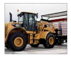
**8-Bar Linkage Design.** This linkage is optimized to maximize reach, specially in applications when manipulating pallets with forks. This provides easiness of operation while approaching the truck to load the pallet
