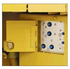
Electric Service Center. Batteries, relay panel and an optional tool box are conveniently located below the left-side access platform. The engine shutdown switch is housed with the relay panel. A compartment integrated into the access platform contains the hood tilt actuation switch, battery disconnect switch and optional jump-start receptacle.
