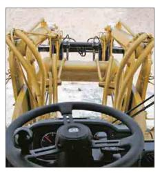
8-Bar Robust Linkage. This linkage provides parallel lift to keep the load level throughout the lift cycle – particularly important when using forks. Parallel lift allows the operator to concentrate on placing the load, instead of retaining it. Visibility to the work tool is excellent. Larger tilt cylinders and a more robust linkage design improve breakout force and overall rackback capability. Rotary sensors for the lift circuit let the operator electronically set detent positions from the cab.
