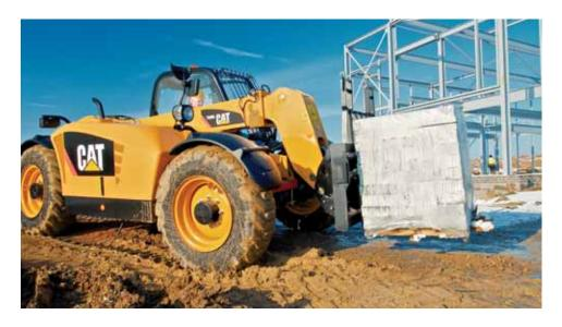
TH-Series machines are equipped with Cat<sup>®</sup> C4.4 engines —74.5 kW (101 hp). A Cat<sup>®</sup> C4.4 DITAAC-ACERT<sup>™</sup> optional engine with 93.1 kW (126 hp) is available for the TH336, TH337, TH406 and TH407. Both engines are certified to Stage IIIA (Tier 3) emission regulations.
