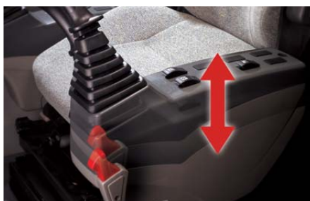
Control stand (Telescopic Function)
