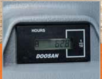
Hour meter (from ground level)
