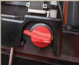
Battery cut-off switch
