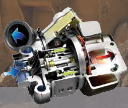
Variable Geometry turbocharger: Provides optimal air flow to the engine combustion chamber under all speed and load conditions, so that exhaust gas is cleaner and fuel economy is improved.
