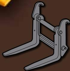
Fork-lift attachment for use with tool carrier
