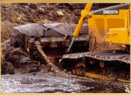
Straight blade of 3.6 cu.m (4.7 cu.yd) used with 2.16 m (85 in) gauge and 940 mm (37 in) track shoes (LGP) is designed for soft, swampy areas. This blade is equipped with hydraulic tilt cylinder to perform efficiently landscaping operations.
