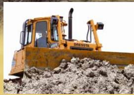
Angle blade of 3.8 cu.m (5 cu.yd) used with STD & LT track frame, is ideal for side-casting, backfilling, cutting ditches or setting a final grade by reducing amount of maneuvering required to do these jobs.
