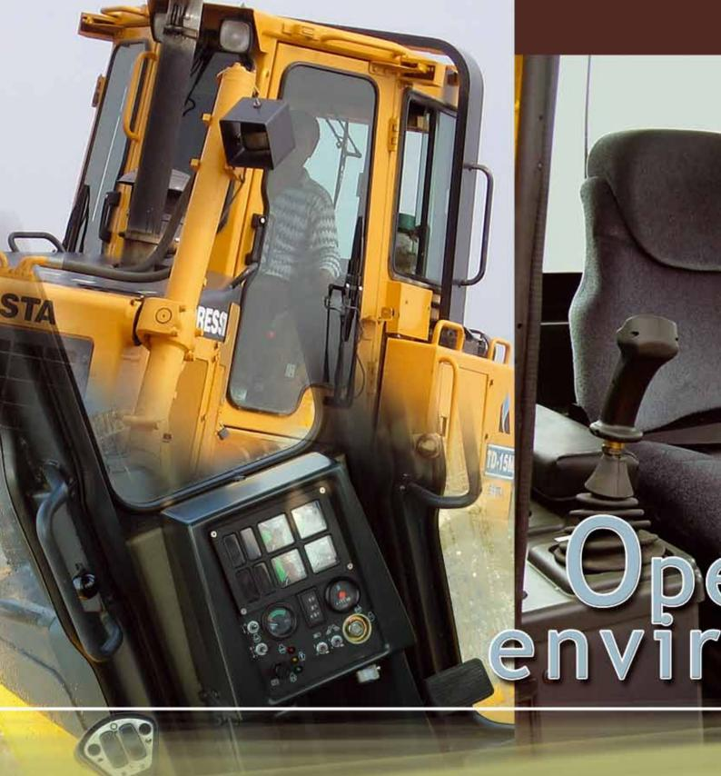
Air suspension type operator's seat is adjustable and equipped with full arm rests and 3 in retractable seat belt.
