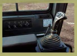
The left hand joystick controls transmission and steering drive for up and down shifting, steering Hi/Lo selection and LH/RH gradual turn. Preset travel speed selection and auto – downshift provide comfortable operation and high productivity without manual downshifting.
