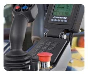
▲ C ontrol panel with valuable information The clear LCD control panel gives operators the information they need. All the gauges are displayed and the operator can change between menus at the touch of a button.
