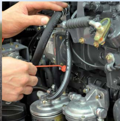
Inspection in a matter of seconds: the large-sized, self-cleaning water filter is located directly behind the tank lock.
