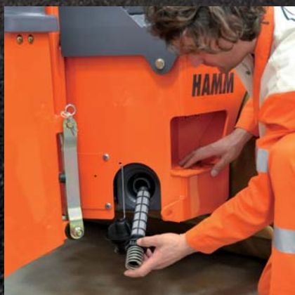
Easily accessible: the well-positioned engine oil dipstick.
