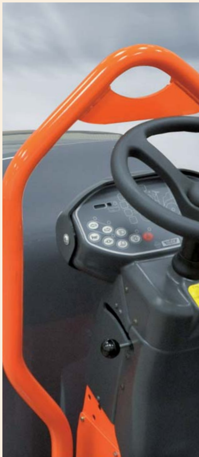
An ergonomically-designed grab handle in the centre of the machine allows rapid and safe access. On the HD 8-12, it also serves as the central suspension point for loading and unloading the machine.
