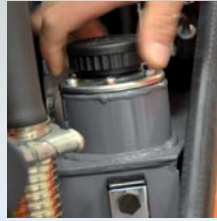
Large filling nozzle for hydraulic oil.
