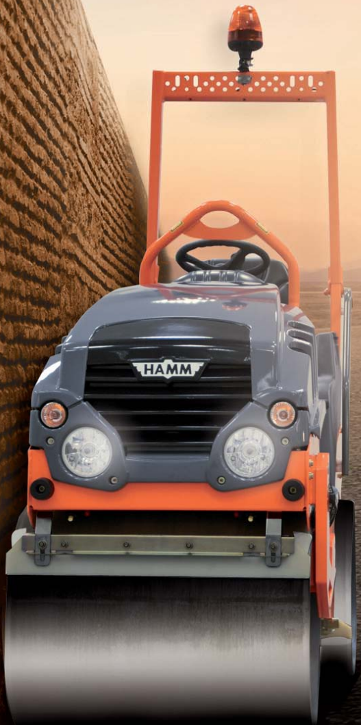
Single-side drum attachment on the HD 8 and HD 10C models ensures complete compaction right up to the edge.
