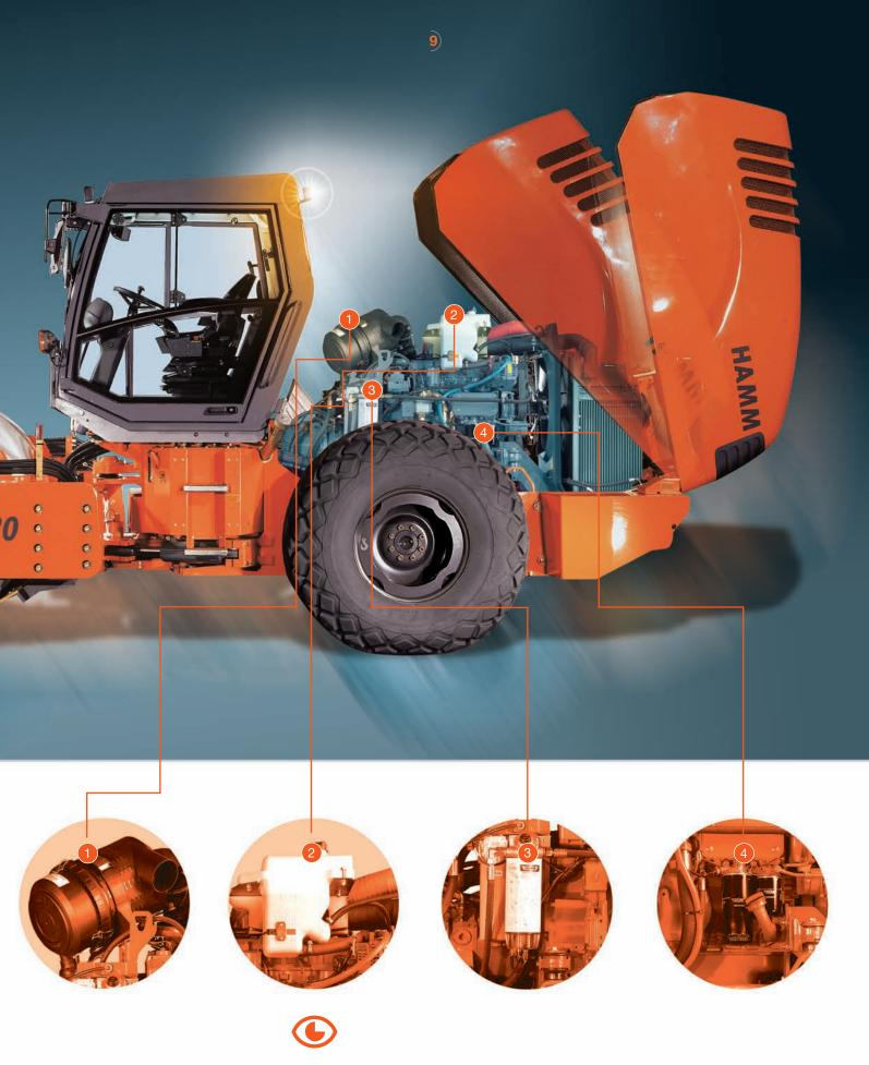
The air filter is easy to exchange by hand.
