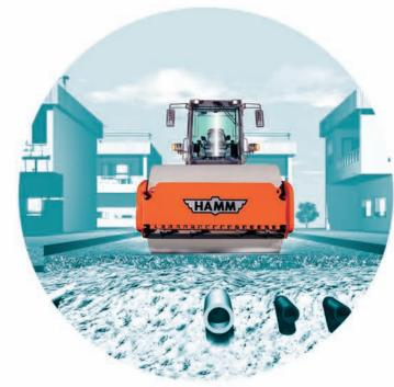
The oscillation can be used, where the vibration cannot be used. Examples? Imagine a very sandy soil - whereupon a vibrating roller is working. The effect: the before compacted sand is again loosened up by the vibrations produced in the machine surrounding field. This is prevented with oscillation.
