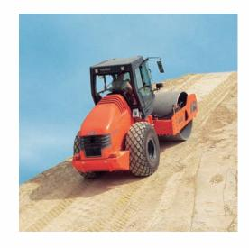
The Hammtronic supervises all engine and roller functions, in particular drive, vibration, oscillation and engine speed. The vibration system and the driving speed are adapted by the electronic engine management to the respective operating conditions. This naturally supports also the operating condition and the life span of the machine. All information is transmitted to the information display and this documents the most current data.
