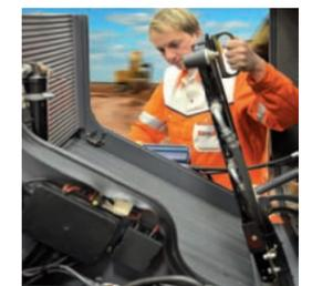
Fold-out condenser for the air-conditioning unit over the engine fluid cooler.
