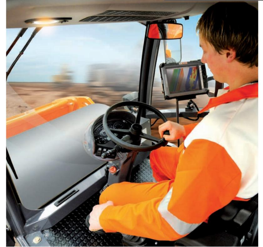
From the cab, the operator has a clear view of the machine and work site. The blind zone in front of the roller drum has an area of less than 1 x 1 m.
