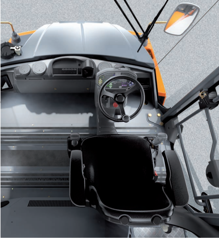
The operator's seat can be shifted to the outer edges of the platform – providing an optimal view of the wheels.
