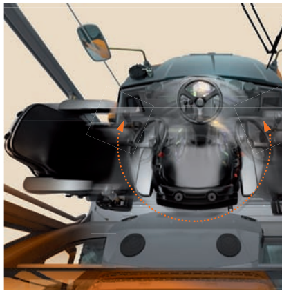
The driving seat can be rotated 90° to the left or right by a single hand movement.
