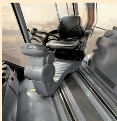
Driving seat and console can be adjusted to any desired operating angle.
