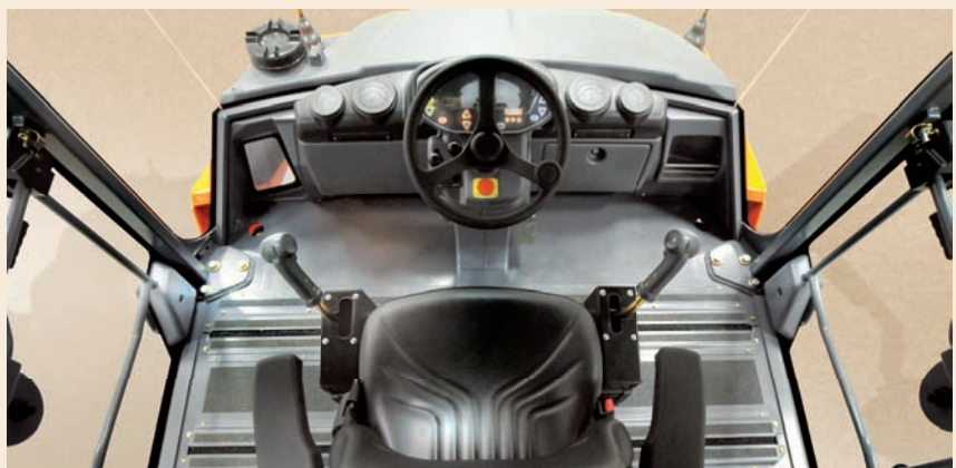
The operating concept of the GRW 280 corresponds to that of a tandem roller. This increases efficiency, since personnel can be flexibly allocated to the operation of either type of machine without having to undergo further on-the-job training.
