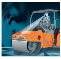
HD 090V - Articulated tandem roller with vibratory and oscillating drum
