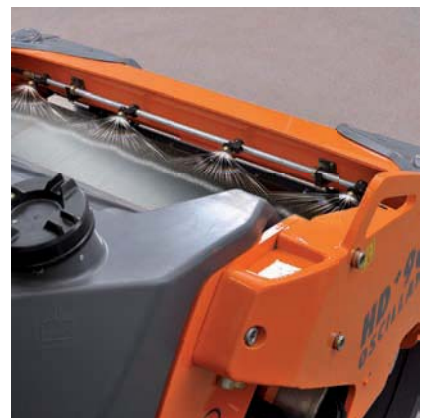
The panoramic cabin and the open upper-frame design allow the sprinkling mechanism to be kept in sight at all times.
