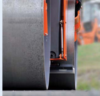
Trouble-free edge pressing thanks to a crab steering mode of up to 170 mm.
