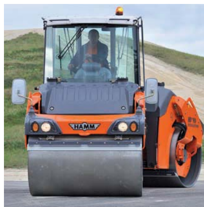
Optimal weight distribution even on narrow turns due to articulated steering.
