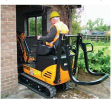
Combination of hydraulically retractable tracks and folding ROPS enables the HO9D to pass through narrow openings with low headroom clearance.
