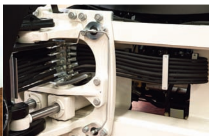
Heavy duty monoblock kingpost carriage with centrally mounted hydraulic cylinders
