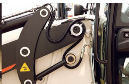
Recessed loader struts and aesthetic hose routing
