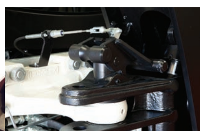
Backhoe boom and slewing lock controlled from inside the operator's cabin
