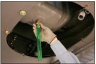
In addition to a pre-filter, dual main fuel filters are provided standard to reduce clogging of the fuel line to the engine.
