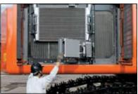
The radiator and oil cooler are laid out in a parallel arrangement, instead of the conventional in-line arrangement. This parallel arrangement is significantly easier to clean around the engine. The air conditioner condenser can be opened for easy cleaning of the condenser and the radiator located behind.
