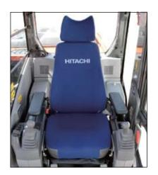
Wide adjustable armrests and a retractable seat belt are included. Short stroke levers allow for continuous operation with less fatigue. The cab is pressurized to keep out dust. Noise and vibrations are kept to a minimum due to the elastic mounts, filled with silicone oil, the cab rests on.
