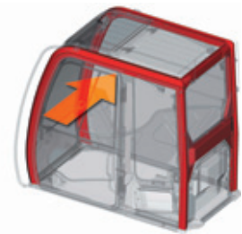
Withstanding load: 2.5-fold increase
