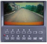
The widescreen colour LCD, teamed up with the rear view camera on the counterweight, provides rearward viewing.
