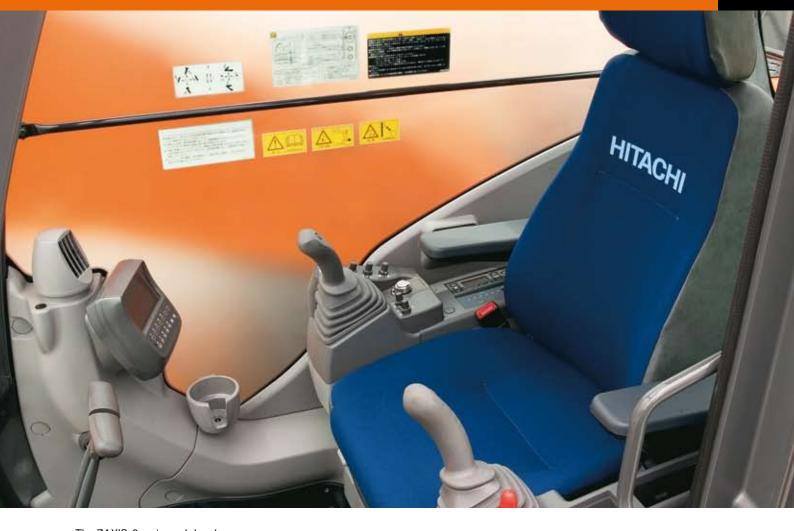
The ZAXIS-3 series cab has been redesigned to meet demands of customers. From the operator's seat the operator has an excellent view of the jobsite. On the widescreen colour LCD monitor the operator can see machine conditions and with the rear view camera, what is behind the machine. Ample legroom, short stroke levers and a suspension seat ensure optimum working conditions. The seat features horizontal, vertical adjustments and has a backrest contoured for comfort, with a HITACHI logo.
