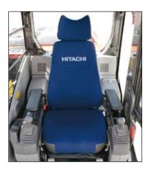
Wide adjustable armrests and a retractable seat belt are included. Short stroke levers allow for continuous operation with less fatigue. The cab is pressurized to keep out dust. Noise and vibrations are kept to a minimum due to the elastic mounts, filled with silicone oil, the cab rests on.
