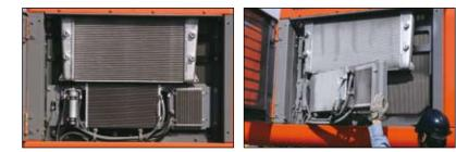
The radiator and oil cooler are laid out in a parallel arrangement, instead of the conventional in-line arrangement. This parallel arrangement is significantly easier to clean around the engine. The air conditioner condenser can be opened for easy cleaning of the condenser and the radiator located behind.
