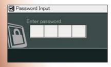
The electronic immobiliser requires the entry of an encryption code to the multifunctional monitor each time when starting the engine to prevent theft and vandalism.
