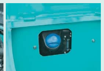
Diesel exhaust fluid tank
