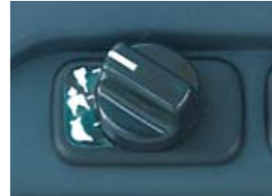
Attachment selector switch
