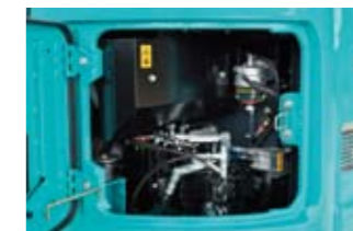
• Firewall separates the pump compartment from the engine
