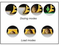
Intuitive selectable load settings Machine control load settings can be adjusted between presets to tailor response to material conditions. From dry loose sandy soils to wet heavy clay materials, system performance can be targeted accordingly.
