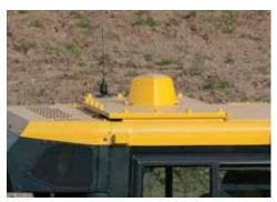
Cab top GNSS antenna No more worries about blade mounted antennas or cables. The cab top GNSS antenna on your D37EXi/PXi-23 reduces risk of damage and theft.
