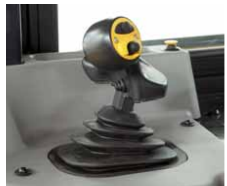
Palm Command Control System (PCCS) with automatic/manual blade control button
