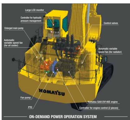
On-demand fan speed and engine output control system ols the rotational speed of the fan ng to the hydraulic oil and coola d varies the engine o in on the fan sneed
