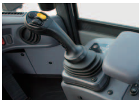
Multi-function lever with optional sliding proportional control for attachments
