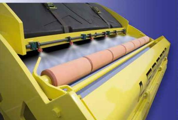
Water is guaranteed for the entire working day. Both plastic tanks prevent the growth of the flora. The capacity of 1000 litres is distributed by means of two interconnected pumps that ensure the continuous operation. A triple filtrate system of different sieves distributes the water to the sprayers. The LEBRERO patented system of foam rollers duplicates the capacity of the tanks. The sprinkling timer regulates the used water flow.
